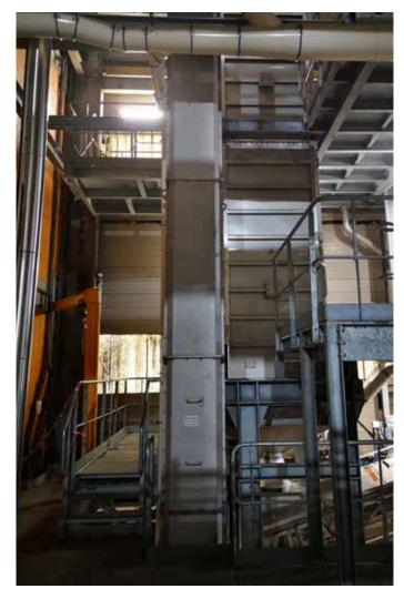
The sugar cooler is static equipment, with the only moving part being the vibrating feeder at the outlet. This device is isolated from the rest of the installation to avoid any transmission of vibrations. Likewise, it has side access doors over the entire height of the plate bank to allow easy cleaning and maintenance.
