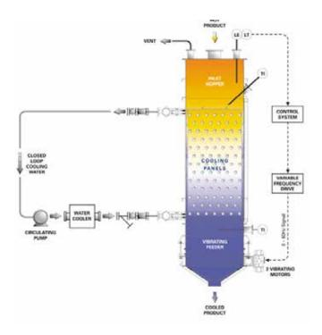
An added benefit to vertical plate technology is its compact size allows for easy integration into existing operations. The exchanger itself takes up very little floor space, typically measuring two meters by two meters and ranging from five to 20 meters tall. (In Bazancourt's case, the height was around 11 meters for a feed rate of 100 tph sugar.)
