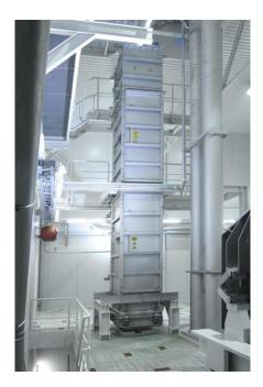
Fig. 1. Sugar cooler at the sugar plant of Lage Germany (Pfeifer & Lange Group).
