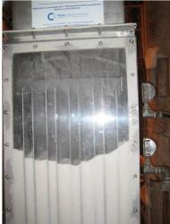
Fig. 2. Pilot unit used for the testing amorphous sugar with Plexiglas window to allow observation of flow.
