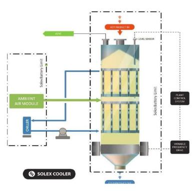
Fig. 4. Schematic of the sugar cooler at Ingenio San Carlos
