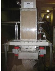
Fig. 3. Pilot unit fitted with a Plexiglas front used to test raw sugar.
