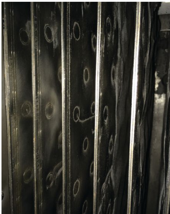
▲ In this green sand application, the image on the left shows caking on the plates that had to be scraped off. The image on the right shows the plates once the material's moisture content was better controlled with the addition of small amounts of purge air.
