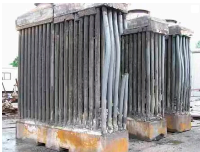
Figure 4: Catastrophic failure in a shell-and-tube heat exchanger.
