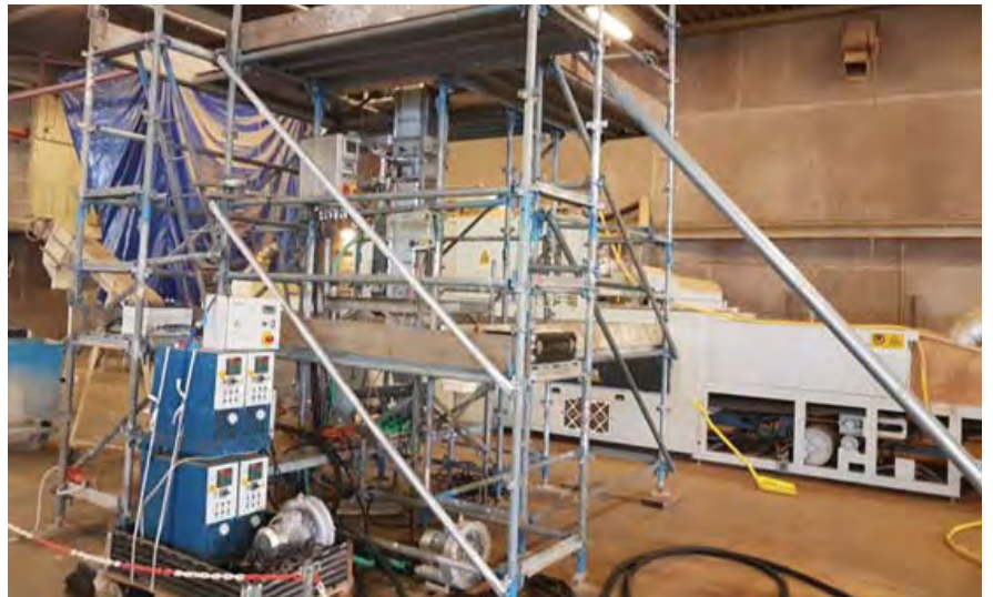
⚡ An on-site pilot test in 2021 validated the thermodynamic design of the MBHE, as well as better understand how the solids would behave in the unit. Courtesy of Solex Thermal Science.
