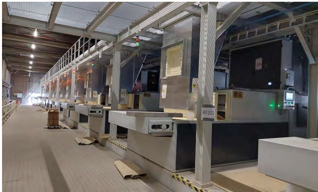
♣ To treat the meal without chemicals while also increasing the nutritional value for its use as or for being processed into the animal feed, Agrifirm a chemical-free process that heats the feed to approximately 130°C through radio frequency waves. Courtesy of Solex Thermal Science.
