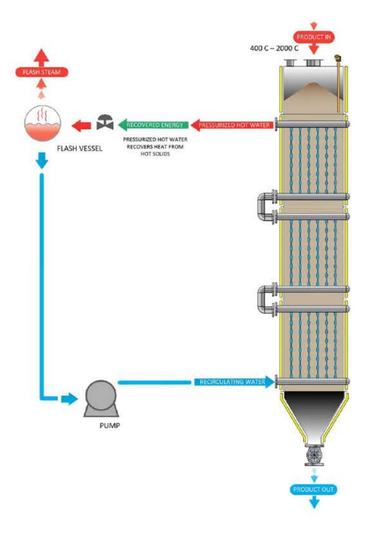
A conceptual energy-recovery loop shows a potential design for cooling high temperature bulk solids such as ash, petroleum coke or graphite.
