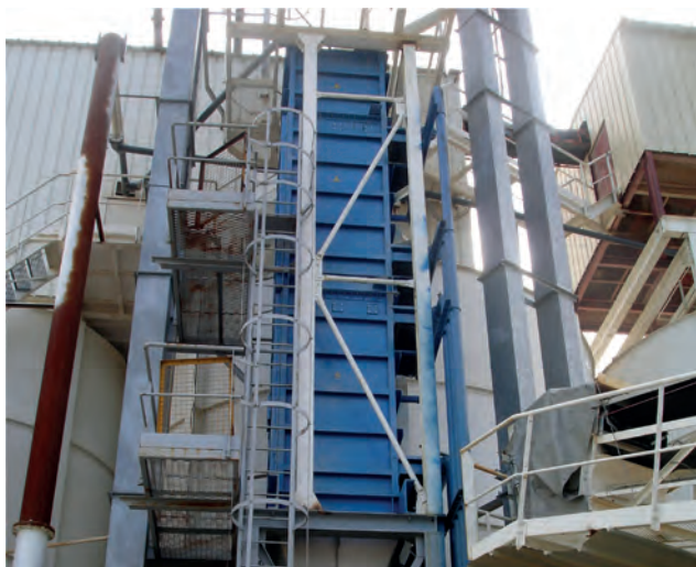
Figure 3. The tower-like design blends the thermal efficiency of plate heat exchange design with the science of uniform mass flow to cool the full range of fertilizers, including urea, ammonium nitrate, CAN, NPKs, MAP, DAP and ammonium sulfate.
