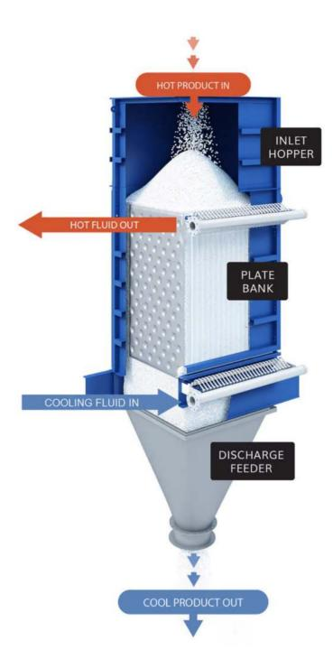
The heat exchange in a moving-bed heat exchanger is realized by conduction across the surface of a series of plates. As the granular solids flow by gravity through the unit, a working fluid flows counter-currently within the hollow plates. A discharge device provides uniform mass flow and, as such, consistent heating or cooling of the solids.
