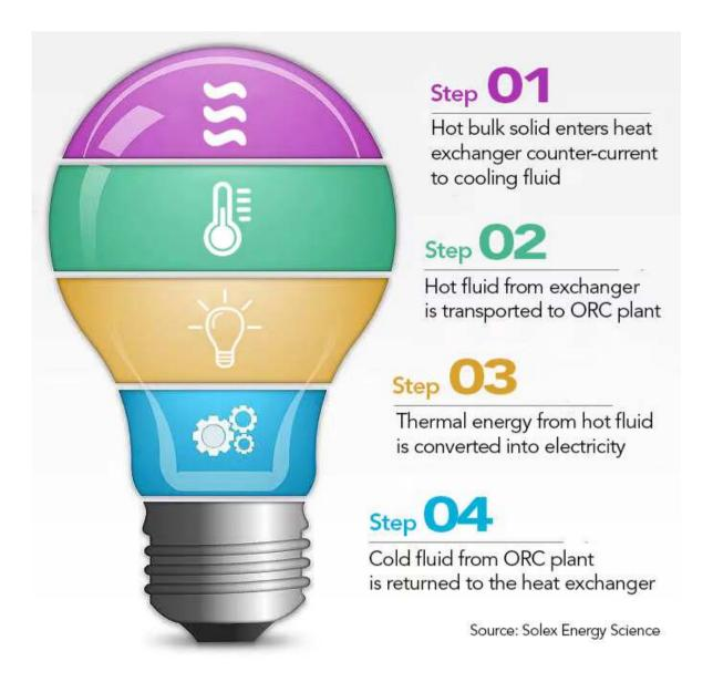
The heat energy in hot bulk solids can be converted into energy through a series of steps.
