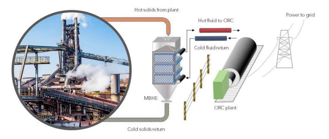
Waste heat to can be converted to electrical power in some high temperature applications using moving-bed heat exchangers and and organic Rankine compression technology.
