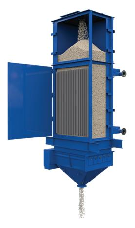
Indirect heat exchangers can consume up to 90% less energy than conventional technologies and in some cases allow for energy recovery loops, increasing overall efficiencies. Since the unit is fully enclosed, there are also no dust emissions. The modular design and small footprint allow for facility retrofits and simple capacity increases. With no moving parts and easy access to individual plates, maintenance costs are lowered, ensuring long term reliable operation.
