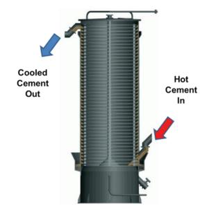
Conventional cement cooling technology has had few advances in the last several decades and are burdened with efficiency and maintenance issues. The conventional design is a cylindrical tube, with an internal ribbon-screw, which elevates the cement and keeps it in contact with the interior surface of the tube. Water is then poured over the exterior tube, cascading down the outside wall, achieving indirect heat transfer, cooling the cement.
