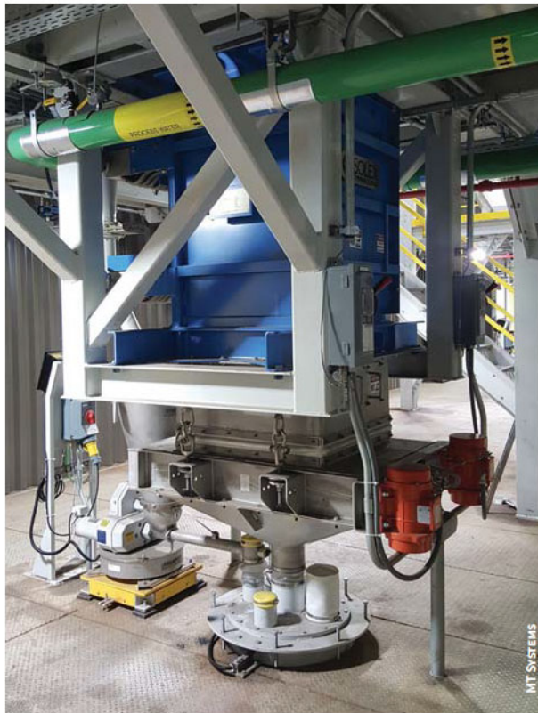
The sand discharge flow rate is managed by a vibratory feeder controlled by the MT Systems control.
