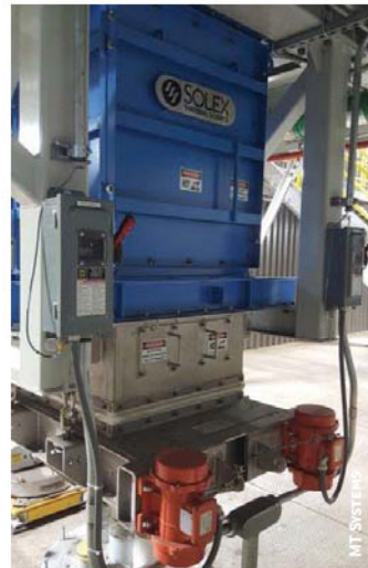
In the Waupaca case, the heat exchanger casing is mounted by standard support brackets below the heat exchanger bank.
