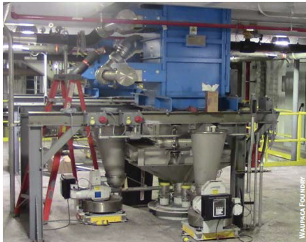
The Solex cooler at Plant 3 in Wisconsin helped Waupaca Foundry to reduce mold core scrap rates by 33% and offset additive costs by 10%.
