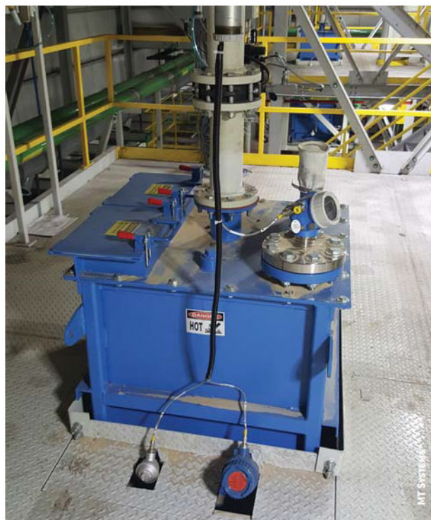
Before entering the heat exchanger, the sand is transported via pressurized air to a receiver hopper that then feeds into the Solex inlet hopper.
