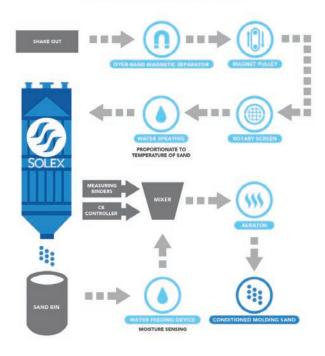
Figure 3. Example of sand conditioning process design
