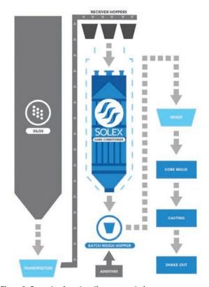
Figure 2. Example of sand cooling process design
