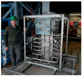
≈ A high-temperature heat exchanger with particulate solids and supercritical CO2, which part of a solar power research project carried out by Sandia National Laboratories in the U.S. Photo credit: Solex Energy Science
