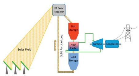
≈ Process diagram of a concentrated solar plant with solid particle energy storage. Photo credit: Solex Energy Science
