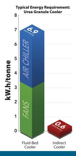
In urea granule applications, indirect heat exchangers consume up to 90 percent less energy than direct-contact alternatives such as fluid beds. (Energy consumption based on estimated operating power requirements, typical for a 3,600 tonnes per day urea plant in a U.S. Gulf Coast location.)
