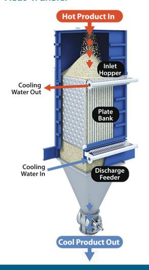
A bank of vertically arranged plates in the exchanger allows free-flowing bulk solids such as fertilizer, sugar and oilseeds to pass through while a separate stream such as water flows counter-currently within the plates. This allows for indirect heating, cooling or drying with the vertical plate heat exchanger. A discharge device at the bottom of the exchanger ensures uniform mass flow and consistent temperature profiles once material exits.
