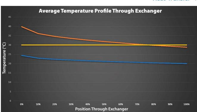
In this cooling application, a product at 104°F (40°C) is fed into the top of exchanger with the target output of 86°F (30°C). At the same time, a fluid at 68°F (20°C) is fed counter-currently into the plates from the bottom. As the product passes through the exchanger, the temperature is uniformly decreased until the product reaches its target temperature.
