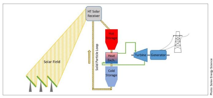
Process diagram of a concentrated solar plant with solid particle energy storage.
