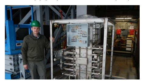
Kevin Albrecht, a mechanical engineer with Sandia National Laboratories, stands next to a particle-supercritical CO2 heat exchanger designed in collaboration with Solex Energy Science.
