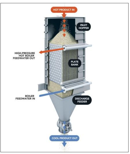
Illustration of a plate unit that is designed to recover waste heat from a bulk solids stream. Installed as an economizer to preheat boiler feedwater.
