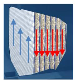
Figure 2 - Exchanger Plate with true counter-flow water
