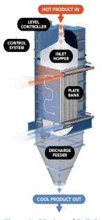
Figure 1 - 3D view of Bulk Solids Cooler
